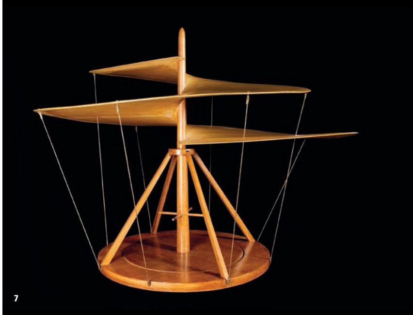
7. This model of the Aerial Screw, designed by Leonardo in the late 15th century, has been seen as the prototype for a helicopter. 167cm x 167cm x 143cm. © Archivio Museo Nazionale della Scienza e della Tecnologia Leonardo da Vinci/Alessandro Nassiri.
